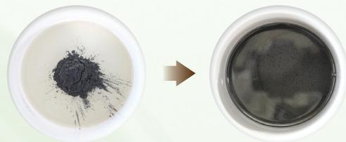
02. Carbon 1g + Silicon 100g(1000RPM + 60 Seconds)
