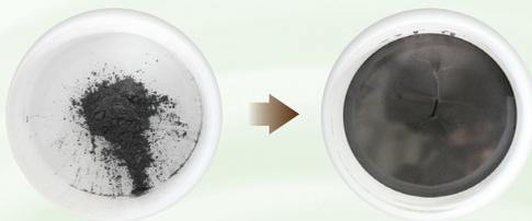
01. Carbon 1g + Silicon 100g(1000RPM + 60 Seconds)
