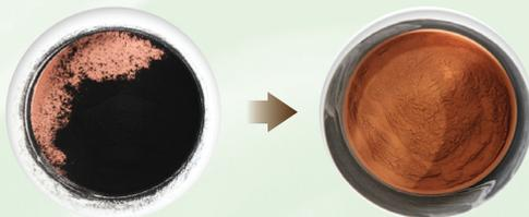
03. Graphene 0.1g + CU Powder 60g(1000RPM + 60 Seconds)
