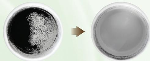
04. Graphene 0.1g + Paint(white) 60g(1000RPM + 60 Seconds)
